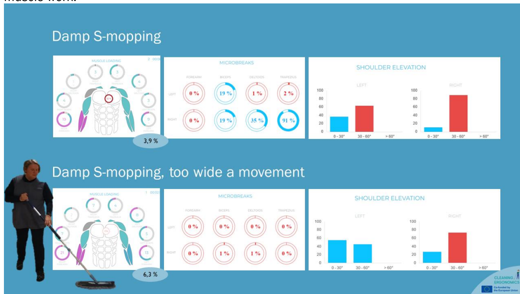
Figure 26: Too wide a working movement increases muscle strain and reduces micro-breaks in muscle work.
